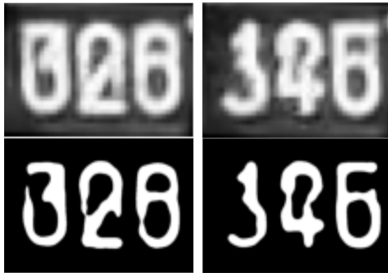
Figure 5: Faulty display images resulting in erroneous OCR readings [31].
