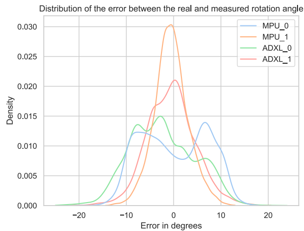
Figure 10: Distribution of the error between the measured and real rotation angle per accelerometer in degrees.
