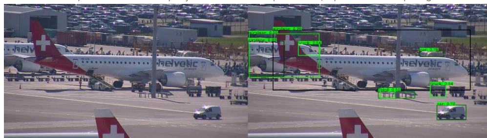
Anonymization followed by object detection at Airport Zurich, Input left and Output right
