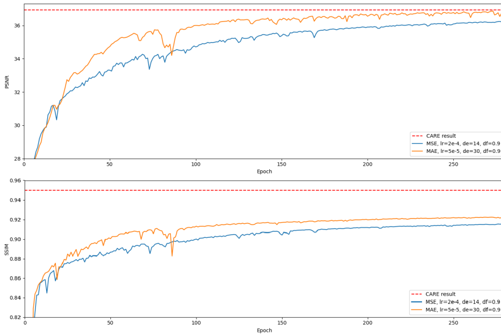
Figure 4.1: PSNR and SSIM: Training of the pre-trained DRUNet network with MAE and MSE loss functions on the Nucleus dataset.
