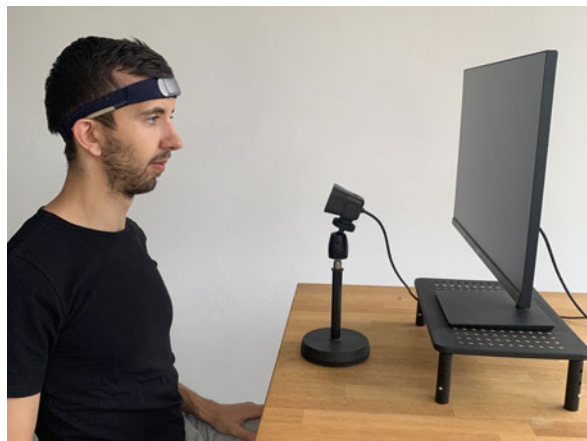
Figure 3.1: Recording setup of the Consumer EEG-ET dataset. The person in the image is the author wearing the Muse S 2 Headband.
