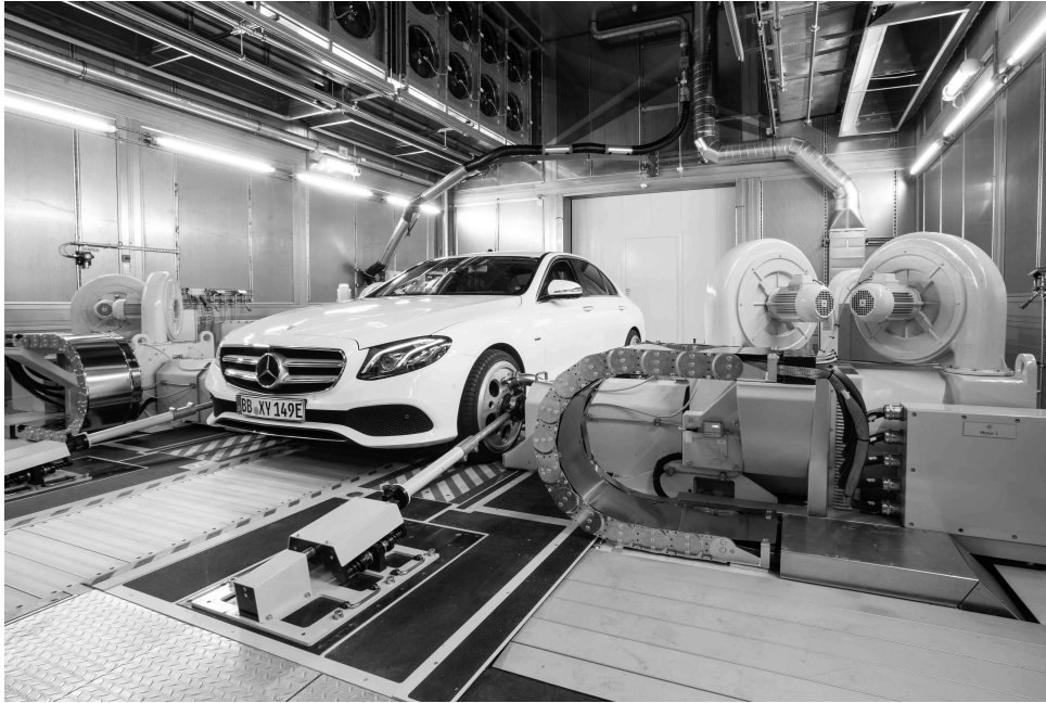
Figure 4.1: KS Engineers R2R test-rig with vehicle mounted. Image from [106]
